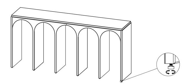
Adjust the leveler for alignment and then Moda Console is ready to use.-
